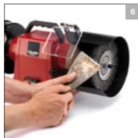
Steel-wire brush for derusting and deburring many types of tools or objects
