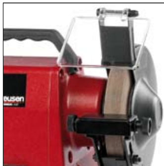
Stable grinding supports fixed on both sides
