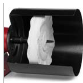
Polishing covers ensure safety during polishing work
