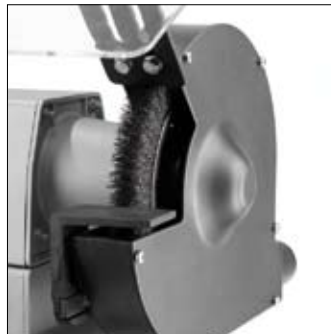
Steel-wire brush fitted inside wheel guard to replace grinding wheel
