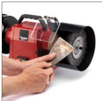
Steel-wire brush for derusting or deburring
