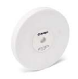
Grinding wheel ø 200 x 25 x 20 mm, grit 60, white art. 700216
